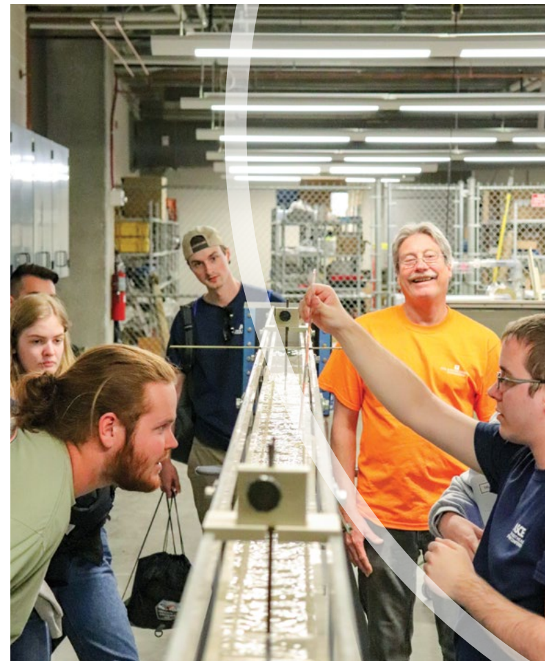
Testing a mechanically stabilized earth wall during the GeoWall competition.
