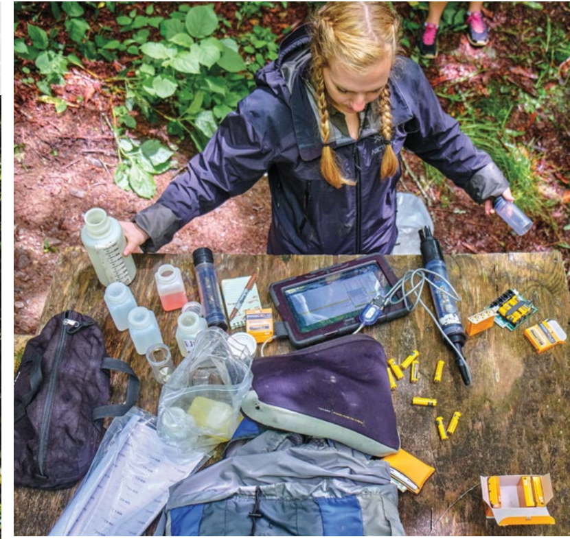
Clockwise from left: Schwartz and graduate student Taylor Blackstone taking data from the open site; Taylor Blackstone tests water samples; bottles are connected to sensors that help monitor groundwater.
